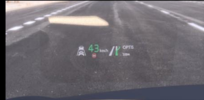
Conventional black coating simulation shows significant screen artefacts in the drivers line of sight
