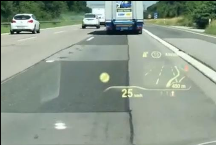
Existing coatings allow distracting sunlight artefacts in the drivers line of sight
